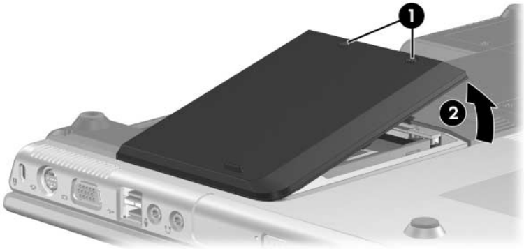
Removing the Hard Drive Cover
